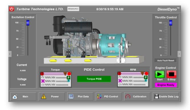
HMI PID Programming Screen
