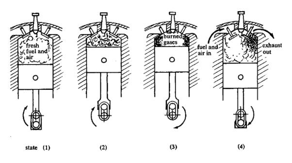
Figure 1-4: The Otto Cycle application in a piston-cylinder device
