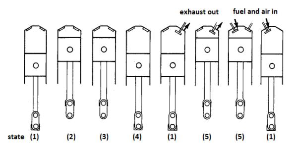
Figure 1-5: Four-stroke Otto Cycle
