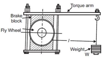
Figure 2-2: Prony Brake (Rope with balance springs) Figure 2-3: Prony Brake (Torque Arm)
