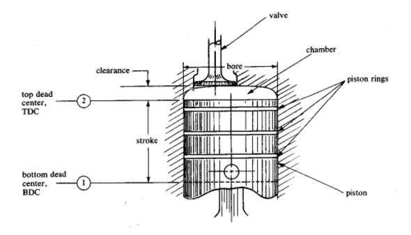
Figure 1-8: Common IC engine parameters
