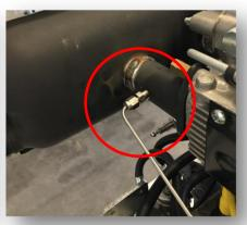
Engine Exhaust Gas Temperature
