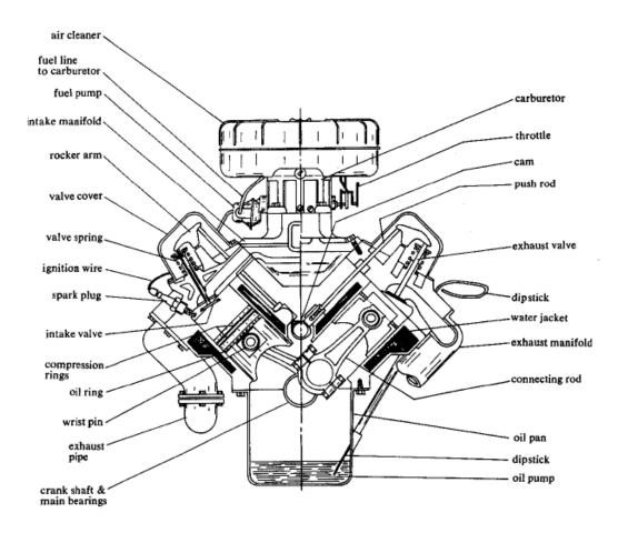
Figure 1-7: Typical internal combustion, spark-ignited engine, V configuration (cross-sectional view)
