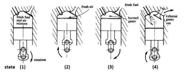
Figure 1-11: Physical Operations of the Diesel Engine
