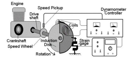
Figure 2-5: Eddy-Current Brake Dynamometer Schematic
