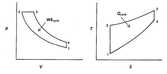
Figure 1-10: Property diagrams for ideal diesel cycle
