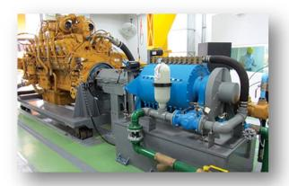
Figure 2-1: Industrial Diesel Dynamometer
