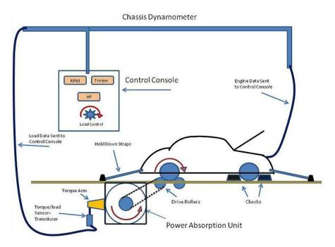
Figure 2-7: Chassis Dynamometer Configuration
