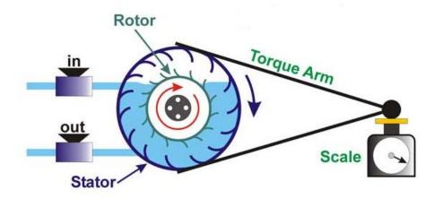
Figure 2-4: Water Brake Dynamometer Schematic
