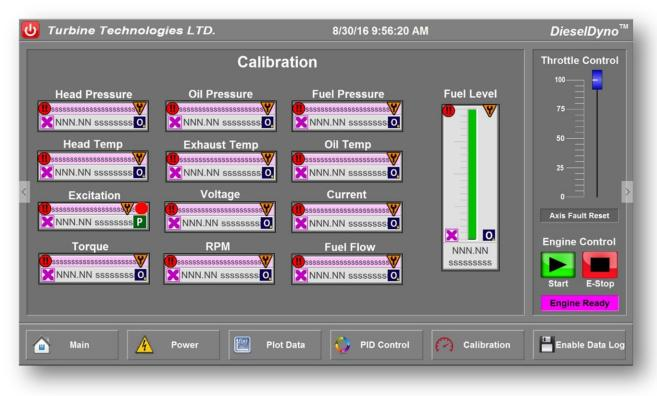
HMI Sensor Calibration Screen
