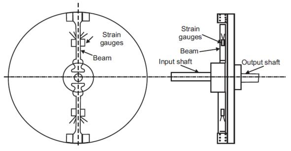
Figure 2-6: Transmission Dynamometer
